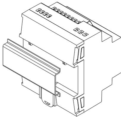
Figure 3: Mounting ALLinBOX Hospitality on DIN rail
