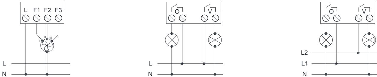
Figure 2: Wiring example (from left to right): three-speed fan, load and open/close valve, load and open/close valve to different phases.
