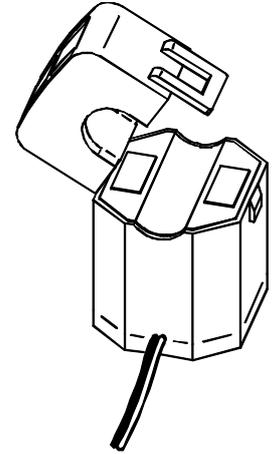
Figure 1. Current Transformer
