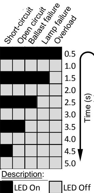
Figure 2. Error notification through DALI channel status LED
