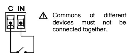
\* In case of using ZN110-DETEC-P sensor, its micro switch number 2 must be in **Type B position**.
