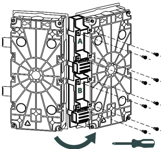
**4** Install the auxiliary parts (A and B) as shown in the figure below.
