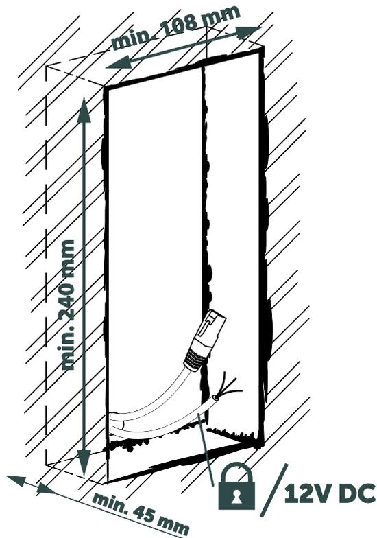
**2** Install the auxiliary parts for the flush-mount assembly.
