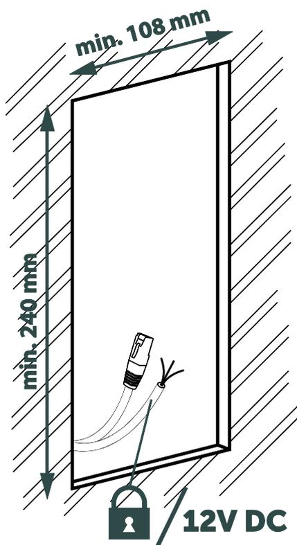
**2** Place the box in the hole, recover the cables and fix the flush-mount box to the drywall by means of the screws that adjust the flaps to the drywall thickness. Please, pay attention to the top orientation mark.
