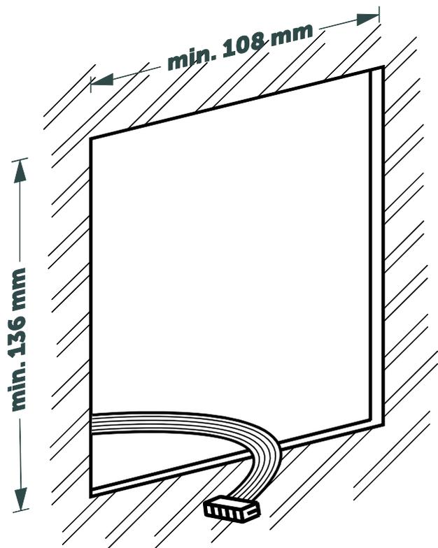
**2** Place the box in the hole, recover the cables and fix the flush-mount box to the drywall by means of the screws that adjust the flaps to the drywall thickness. Please, pay attention to the top orientation mark.
