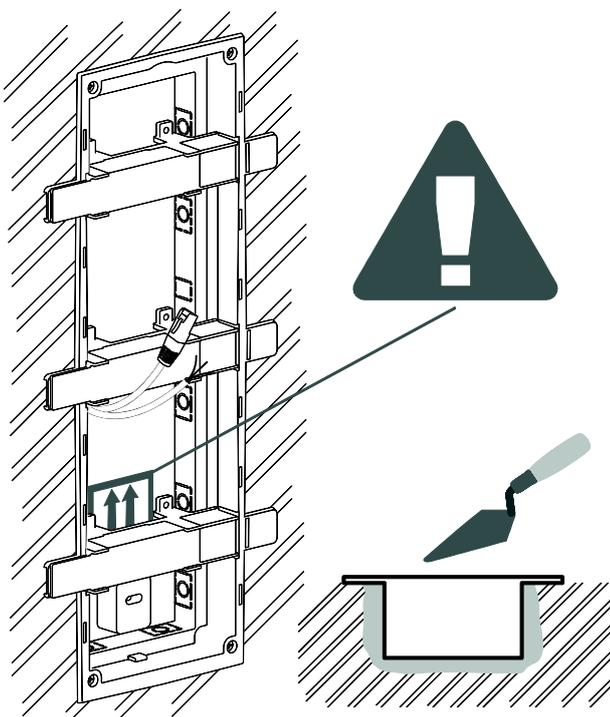
**4** After the setting time, please remove the auxiliary parts and cut the flaps.
