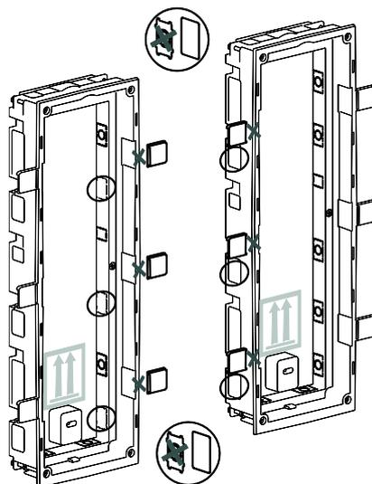
**3** Assemble the boxes by using the auxiliary parts (A and B) and the tube-shape parts. Fix it with the screws.
