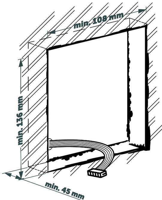
**2** Fix the box by means of mortar, adhesive cement or any other similar construction material. Please, respect the top orientation mark and recover the cables.
