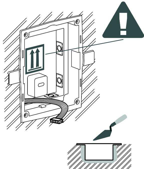
**3** After the setting time, please remove the auxiliary parts and cut the flaps.
