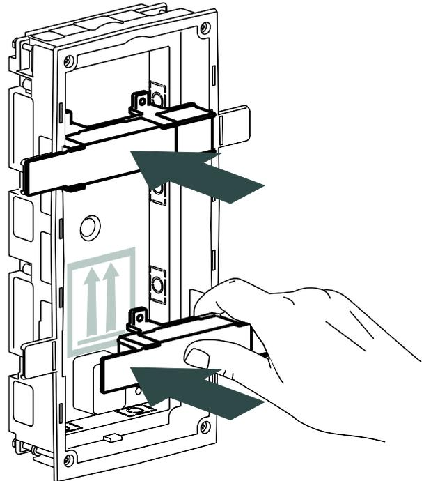
**3** Fix the box by means of mortar, adhesive cement or any other similar construction material. Please, respect the top orientation mark and recover the cables.
