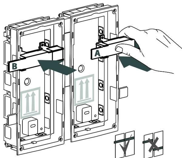
**5** Fix the box by means of mortar, adhesive cement or any other similar construction material. Please, keep the top orientation mark and recover the cables.
