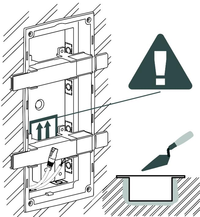
**4** After the setting time, please remove the auxiliary parts and cut the flaps.
