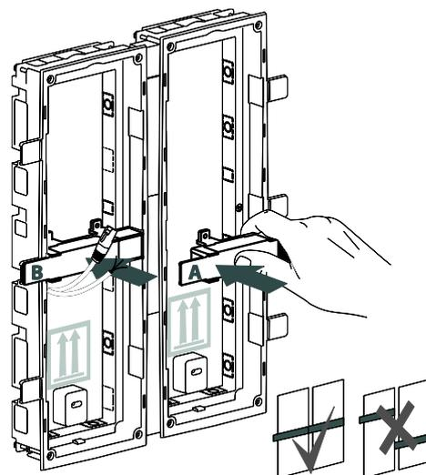
**5** Fix the box by means of mortar, adhesive cement or any other similar construction material. Please, keep the top orientation mark and recover the cables.
