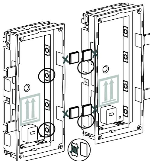
**3** Assemble the boxes by using the auxiliary parts (A and B) and the tube-shape parts. Fix it with the screws.
