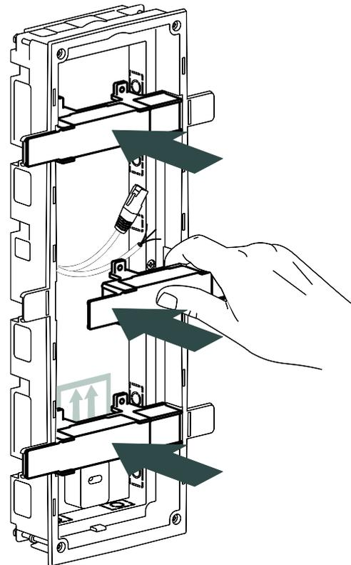
**3** Fix the box by means of mortar, adhesive cement or any other similar construction material. Please, respect the top orientation mark and recover the cables.
