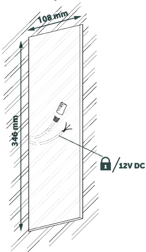
**2** Place the box in the hole, recover the cables and fix the flush-mount box to the drywall by means of the screws that adjust the flaps to the drywall thickness. Please, pay attention to the top orientation mark.
