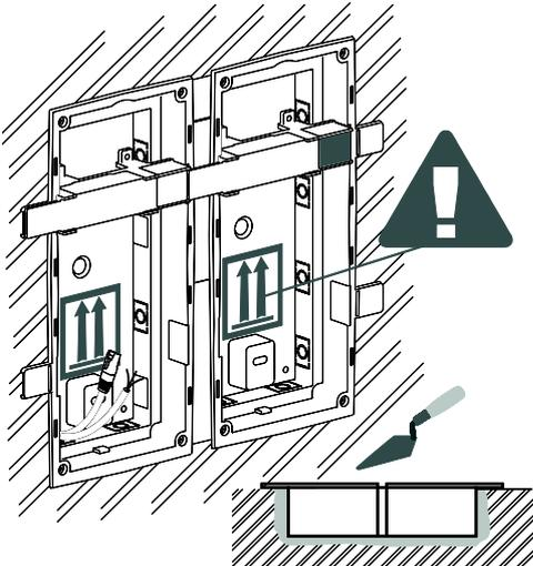
**6** After setting time, please remove the auxiliary parts and cut the flaps.
