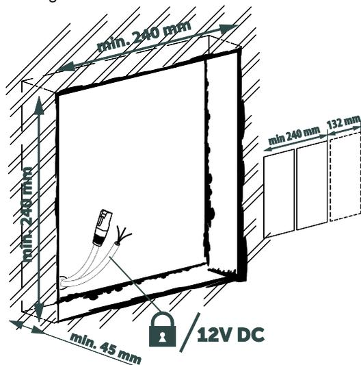
**2** Cut the flaps and open the marked holes in the adjoining sides of the boxes.
