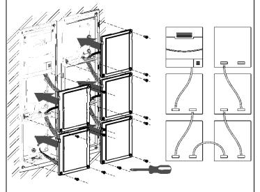
**4** Make the connections of the basic unit and prepare the additional modules. Pass the bus cables through the gaps.
