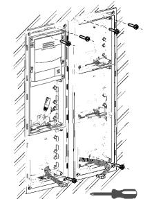
**5** Interconnect the additional modules with the bus as indicated in the schema and then, fix the additional modules with the supplied screws.
