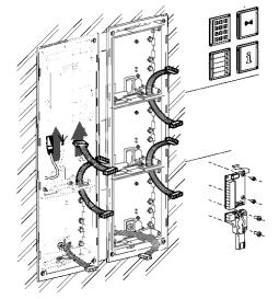
6 Place the frames and fix them by using the supplied Allen key.\*
