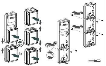
3 Fix the assemblies to the flush-mount boxes with screws.
