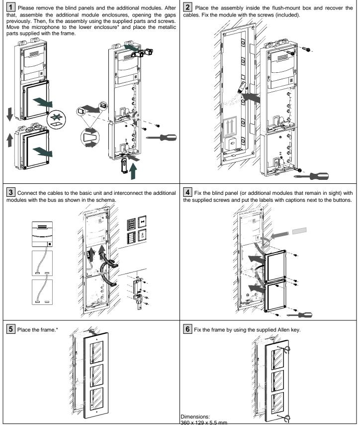
\*In case of acoustic deficiencies, Zennio may supply a modified frame for whose installation step number 1 should be ignored. In such case, though, it is essential that the microphone remains properly connected.
