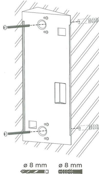
**3** Fix the basic module to the backplate by means of the screws supplied with the first one.
