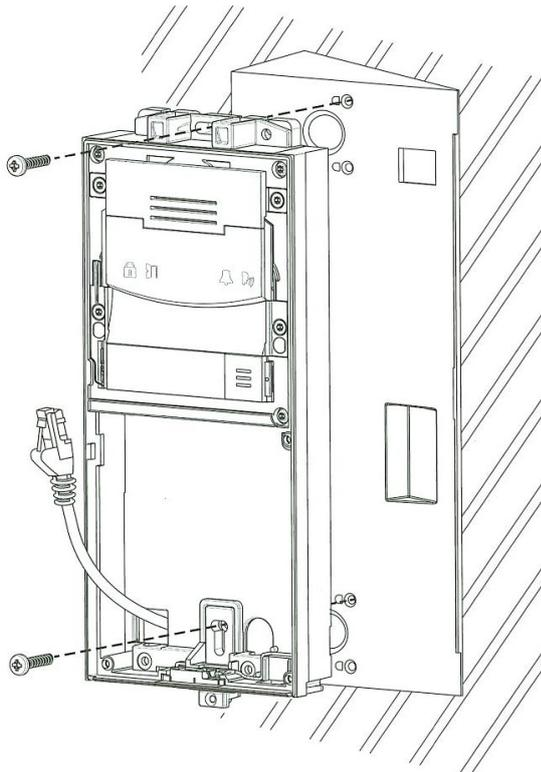
**4** Place and fix the Surface Frame ZVP-CB2M with the Allen key.
