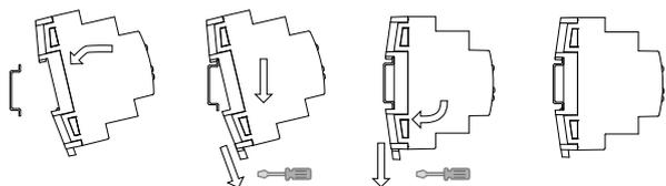
Removing HeatingBOX 230V 4X from DIN rail:
