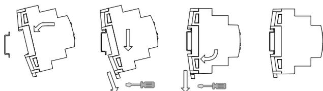
Removing HeatingBOX 24V 4X from DIN rail:
