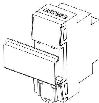
Figure 3: Mounting HeatingBOX 24V 4X on DIN rail
