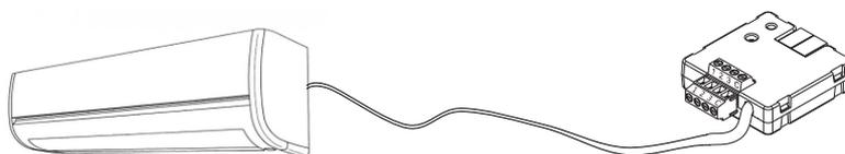
Figure 2. Wiring KLIC-DD3 to a Daikin device
