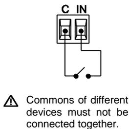
\* In case of using ZN110-DETEC-P sensor, its micro switch number 2 must be in **Type B position**.
