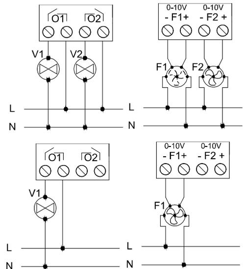
Figure 2: (From left to right and from up to down) Wiring examples for two valves, two fans, one valve and one fan.
