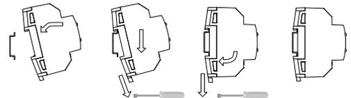
Removing MAXinBOX FC 0-10V FAN from DIN rail:
