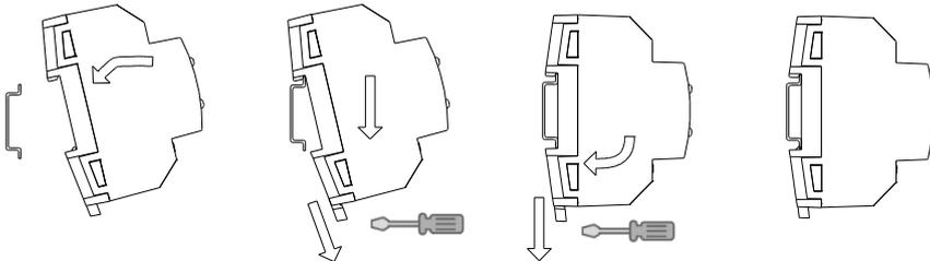
Removing MAXinBOX SHUTTER 4CH v2 from DIN rail:
