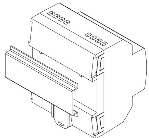
Figure 3: Mounting MAXinBOX SHUTTER 4CH v2 on DIN rail
