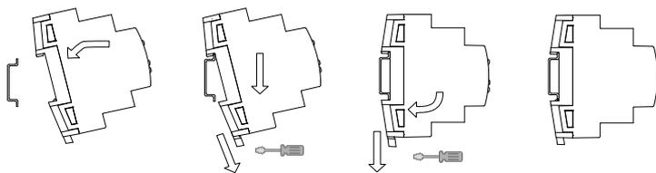
Removing MINiBOX 0-10V X3 from DIN rail:
