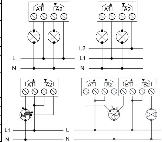
Figure 2: Wiring example (from left to right, and up to down): 2 loads, 2 loads connected to different phases, shutter and fan coil
