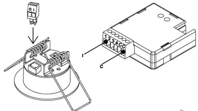
Make a circular hole with a diameter equal to 40 mm .
