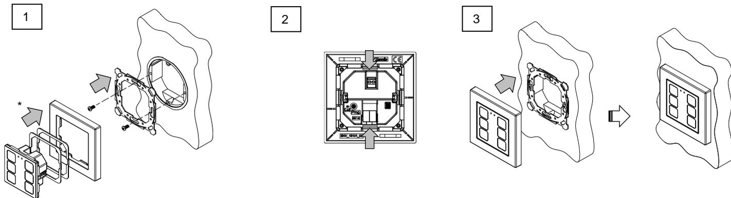
\* (Optional) Insert the metallic levelling plate/s so the device stays at the desired level.
