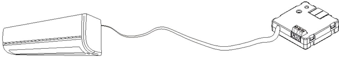
**Figure 2.** Connecting KLIC-MITT v2 to the A/C unit
