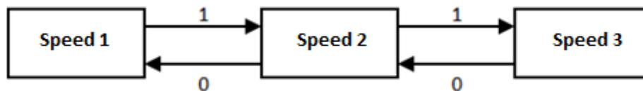
Figure 13. Non-cyclical fan step control (three fan speeds *without automatic mode*).
