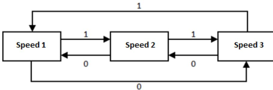
Figure 12. Cyclical fan step control (three fan speeds *without automatic mode*).
