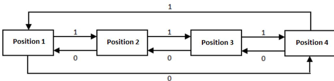
Figure 15. Cyclical flap step control (4 positions and no swing function)
