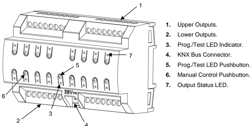
Figure 2. Element Diagram for MAXinBOX 16 v3
