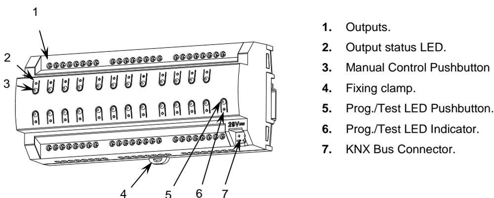
Figure 1. Element Diagram for MAXinBOX 24.
