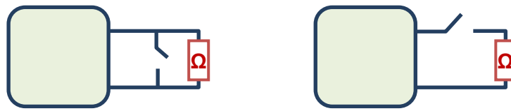
Abb. 4. Linkst: NO (paralleler Widerstand). Rechts: NC (Widerstand in Reihe).
