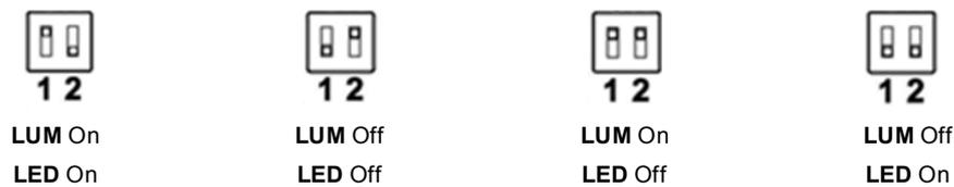
Figure 4. Positions of the Double Micro-Switch
