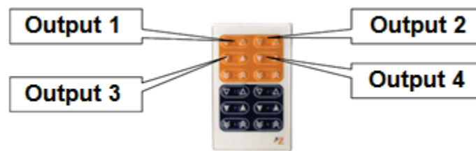
Figure 3 Controlling the outputs from the IR remote
