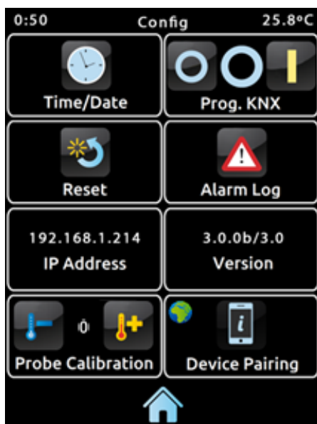
Figure 89 Configuration page with Device Paring enabled.
