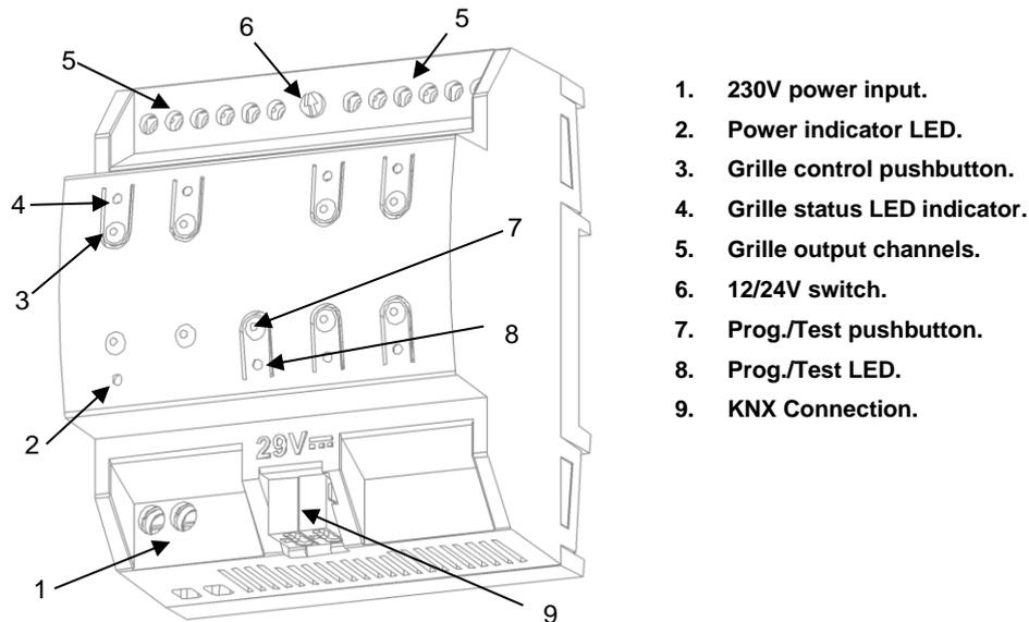
Figure 2. Element diagram (ZoningBOX 6)
