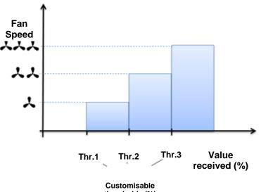
thresholds (%) Figure 16. Thresholds, value received and fan speed
