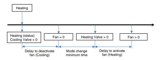
Figure 9. Delay for fan activation/deactivation.
