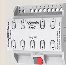
HeatingBOX 230V 8X * (Ref. ZCL-8HT230) Heating actuator for up to 8 outputs 230VAC.
