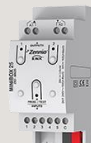
MINiBOX 25 (Ref. ZIO-MN25) Multifunction actuator with 2 outputs (16A) and 5 analog-digital inputs
